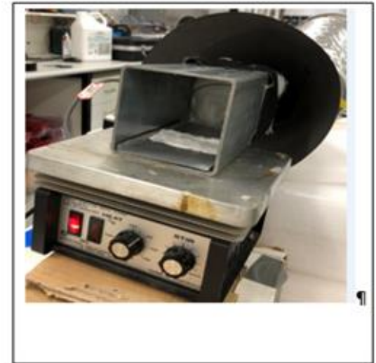
Figure 3: Formaldehyde vapour Generation (heating Paraformaldehyde on hotplate)
