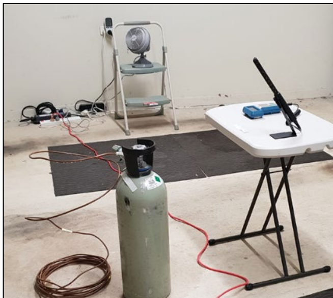
Measuring air exchange in test room using the carbon dioxide decay method
