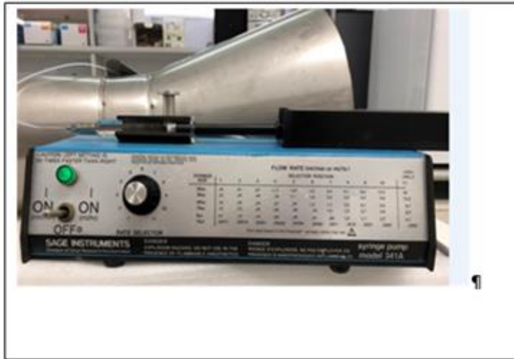
Figure 2a: Syringe pump
