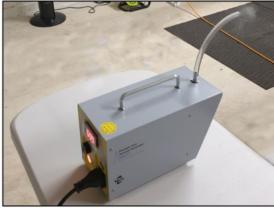
Portable test aerosol generator (note aerosol on top right of image)
