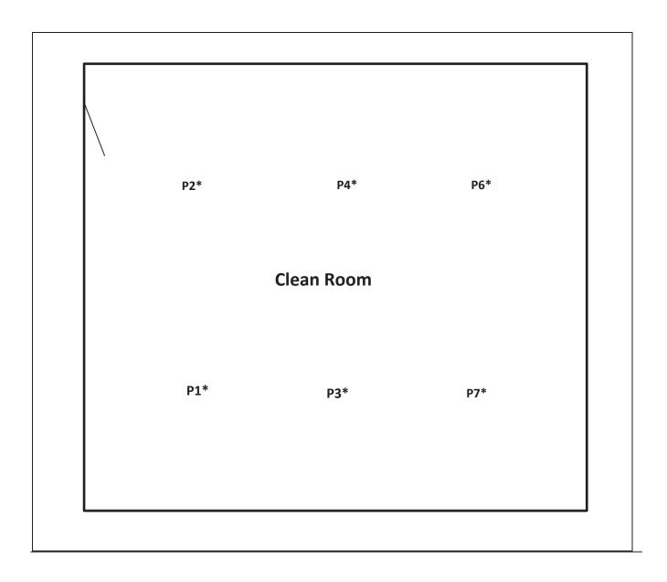
Comment: Pass and/or Fail decision are based on the estimated probability that the calculated result is within the limited specified in the requirements for ISO 14644.1. A pass result is reported when the estimated probability is greater than or equal to 95% of the specified limit.
